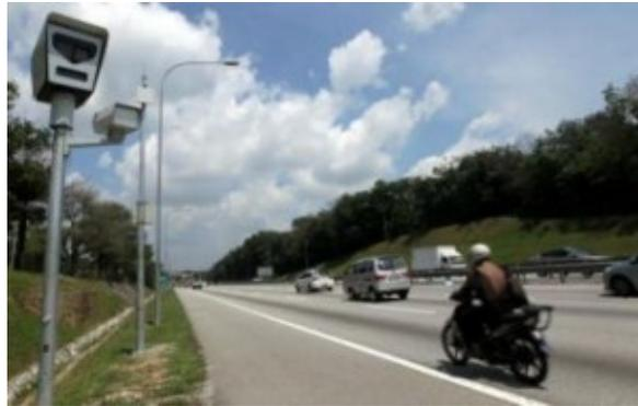
Automated Enforcement System (AES) seen here is a speed camera placed at several locations along highways to discourage speeding (photo from [aesdetector.blogspot.com](http://aesdetector.blogspot.com)).
