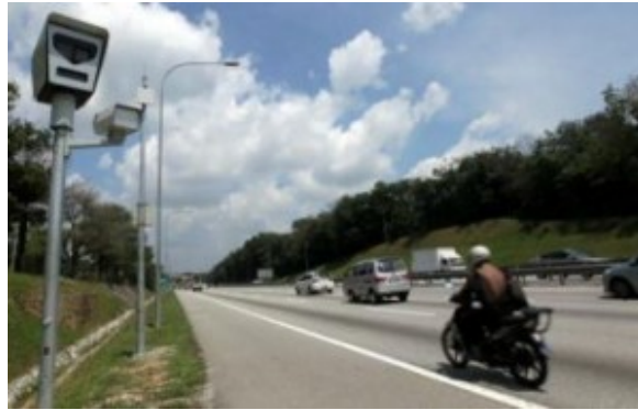
Automated Enforcement System (AES) seen here is a speed camera placed at several locations along highways to discourage speeding (photo from aesdetector.blogspot.com ).
