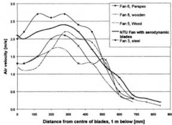
All ceiling fans display the so-called humped airflow profile, where airflow velocity increases from the fan center before reaching maximum (i.e., hump) at about midway of the blade length, then decreases farther along the blade length (Schmidt and Patterson, 2001).
