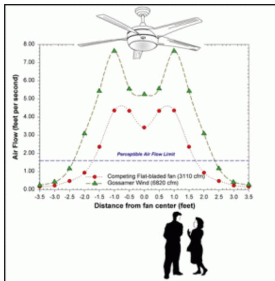
The humped airflow profile means if we stand directly under the fan center, we would feel little airflow
