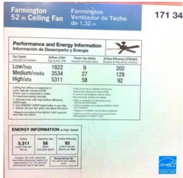
Compulsory labelling. All ceiling fans sold in Malaysia should come with information about the fans' performance: their CFM, power consumption, and efficiency, so that we can make intelligent comparisons between fans (photo from [www.energyvanguard.com](http://www.energyvanguard.com)).
