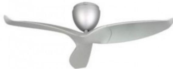
Aeratron ceiling fan has won awards for its very quiet operation and high energy efficiency. Only with three blades but with careful design (such as using winglets and twisted blades), this fan, at top speed, generates about 5,800 CFM, consumes about 15 W, and has an outstanding fan efficiency of 383 CFM per W (photo from [aeratron.org](http://aeratron.org)).
