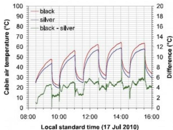
Levinson and associates confirmed that darker coloured cars are warmer than lighter coloured cars. Shown here are car cabin temperature fluctuations during heating (car aircon off) and cooling (car aircon on) cycles for a black and a silver car. "Black-silver" denotes the difference between the
