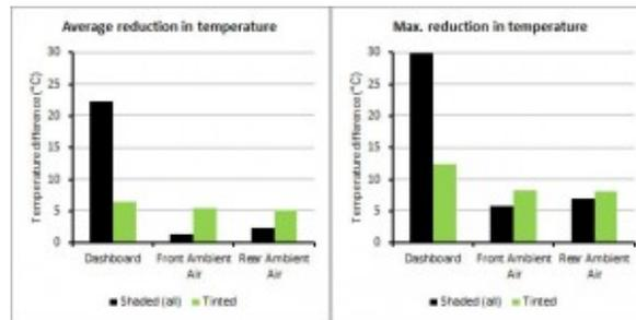
Average and maximum reduction in temperature by sunshade and tint compared to without any cooling methods (baseline) (redrawn from Jasni and Nasir, 2012).
