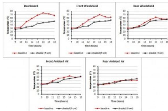
Car cabin does not warm uniformly, where the dashboard experiences the highest warming. Sunshade (placed behind the front windshield) lowered the temperature of the dashboard and front ambient air, but the sunshade had a less cooling effect on the rear windshield and rear ambient air (redrawn from Al-Kayiem et al., 2010).
