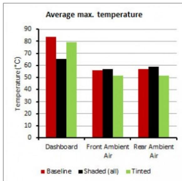
Average maximum temperature in the car cabin. Baseline is that without any car cooling methods (redrawn from Jasni and Nasir, 2012).
