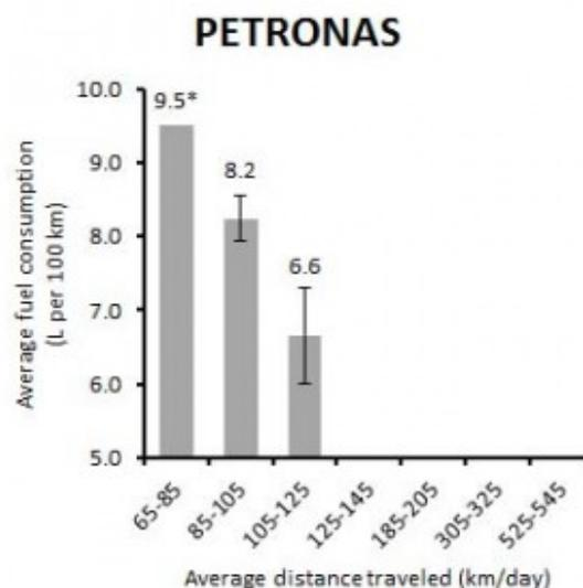
Fig. 3. The fuel consumption for the old formulation of Petronas (note: asterisk denotes insufficient measurements for confidence)
