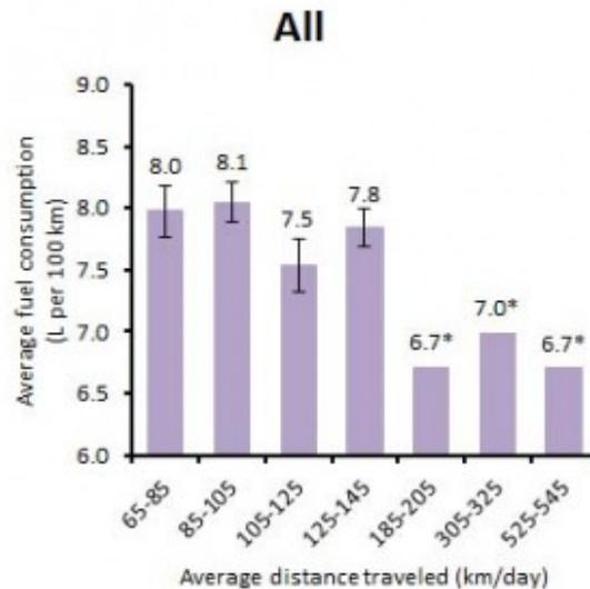
Fig. 1. Fuel consumption for several distances traveled per day (note: asterisks denote insufficient measurements for confidence interval calculation)
