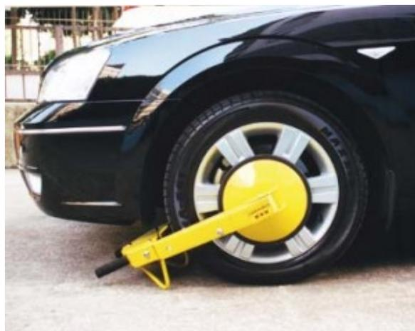
Tire clamp/lock is a good way to prevent towing of your car. If the front tire is locked, ensure you park your car facing towards a wall or obstacle. If the rear tire is locked, then park so that your car rear faces the wall or obstacle. (photo from [www.easybizchina.com](http://www.easybizchina.com))
