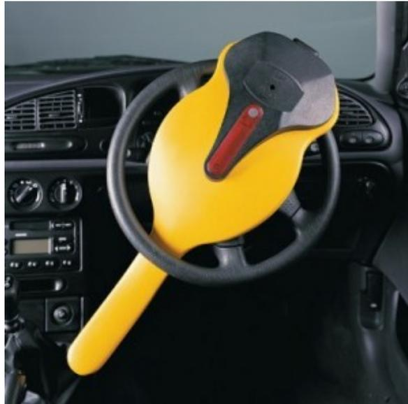
Stoplock Ultima covers the hub and cannot be removed even if the steering wheel is cut, provided the lock is installed correctly. Disadvantages: heavy and expensive and does not fit all wheels. No longer sold in Malaysia. (photo from [www.cartuningparts.co.uk](http://www.cartuningparts.co.uk))
