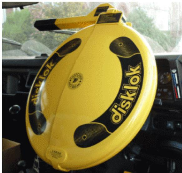
Disklok covers the steering hub and wheel completely. Disadvantages: expensive and heavy. However, it comes in three sizes to fit different steering wheel sizes. (photo from
