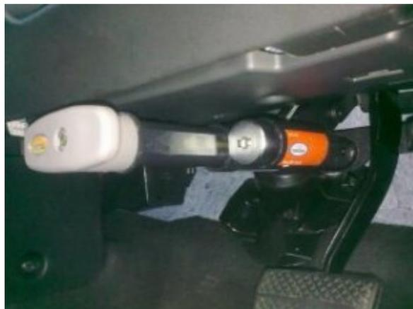
Locktech pedal lock (photo from [static.lowyat.net](http://static.lowyat.net))
